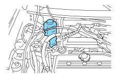
Check the washer fluid whenever you stop for fuel. The reservoir is highlighted with a  $\overleftrightarrow{\Box}$  symbol.
